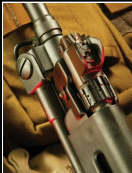
The FAL has a variable gas port by the front sight. If the action gets gunked up, open the port to give the piston more gusto.
