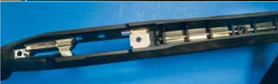
The full-length aluminum bedding block of the Hogue stock extends through the length of the fore-end and offers support in the critical recoil lug area.
