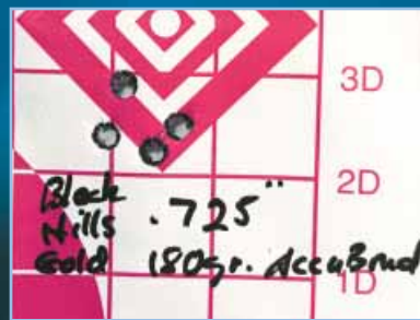
The best group achieved on the author's first outing measured .725-inch. It was fired with Black Hills loads using Nosler 180-grain AccuBonds.
