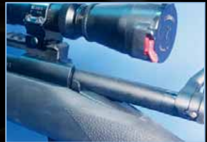
The classic Model 70 action should be familiar to many readers. The bolt stop/release is visible here at the rear of the receiver.
