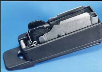
The detachable box magazine is shown while still attached to the floorplate.
