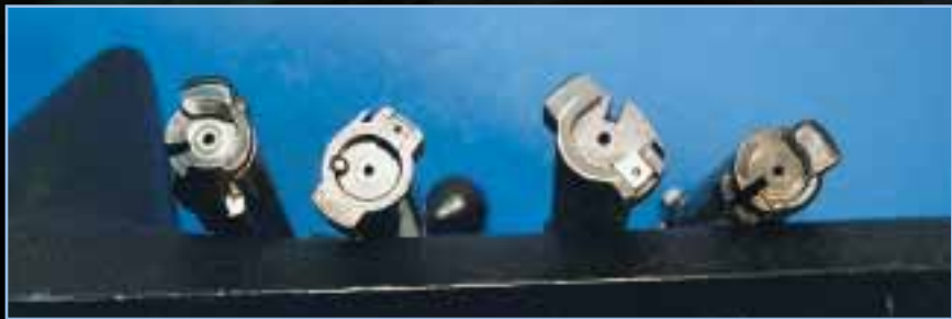
A study in bolt faces (from left): Pre-1964 Model 70, post-1964 Model 70, Controlled Round Push Feed Model 70 (as used on the PBR), Mauser Model 98.
