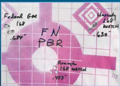
Here are three excellent groups fired with 168-grain match loads from three different makers. The four-shot group fired with the Remington loads measures a scant .453-inch.
