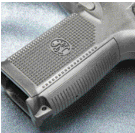
The FNP-45 comes with two interchangeable backstraps. It is shown here with the arched version, which fit the author's hand just fine.
