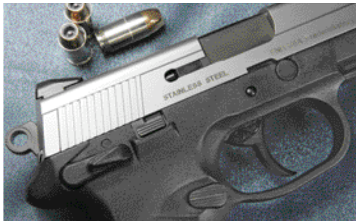
All the FNP-45's controls except the takedown are truly ambidextrous. Rodriguez would have preferred a smaller decocker and taller mag release.
