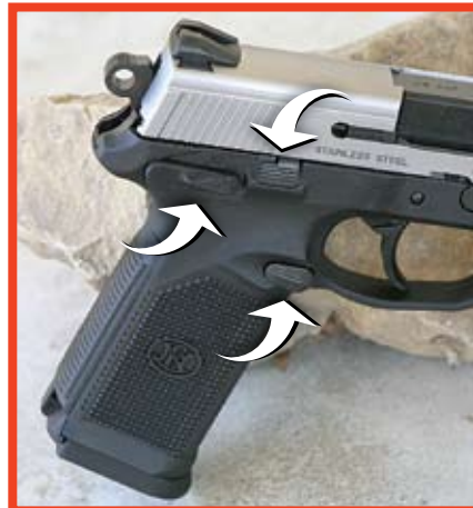
From the rear of the frame, we have the ambi decocking lever, ambi slide release lever and ambi mag release button.
