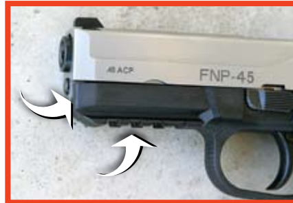
The dustcover is formed as an M1913 accessory rail. The front of the slide is beveled to easy reholstering.
