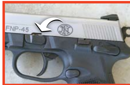
On the right side, the disassembly lever is right above the trigger. Turn it ninety degrees clockwise with the magazine out and the slide locked back, and the slide can be removed for maintenance.
