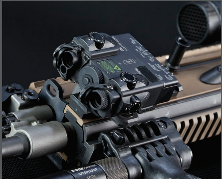
Lasers Devices DBAL-A2 is standard US military issue and combines laser pointer and illuminator in either visible or infrared (IR).
