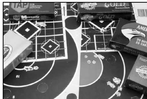
Representative three-shot groups fired at 100 yards with Burris target scope set on 20x and rifle supported by a Harris bipod.
