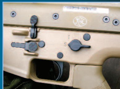
This photo offers a good view of the SCAR's safety, bolt release, and ambidextrous mag release.
