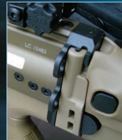
There are dual sling-mounting points at the rear of the SCAR's receiver.
