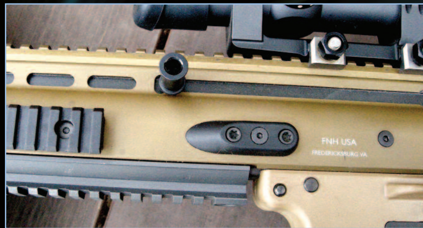
The SCAR's cocking handle may be switched to suit the operator. Here it is installed for operation by the left hand.
