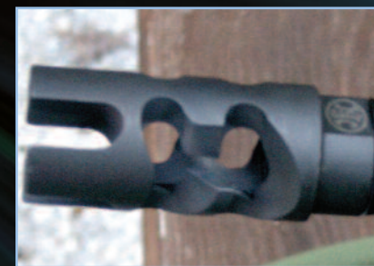
The SCAR features a four-pronged compensator/muzzle brake.
