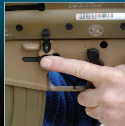
When firing from the left-side shoulder the forefinger can readily work the ambidextrous mag release button.
