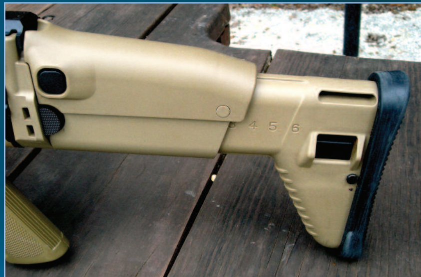
Here the SCAR's stock is set in the position Thompson prefers—the "3" position. The "square" button at the front of the stock releases the cheek piece for adjustment, and the "half circle" button releases the stock so it may be folded. The "switch-type" button at the rear of the stock allows it to be adjusted for length.
