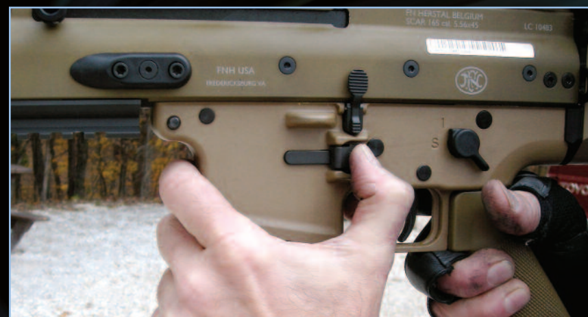
The support-side hand may be used to quickly change a magazine by depressing the release button and pulling on the magazine.
