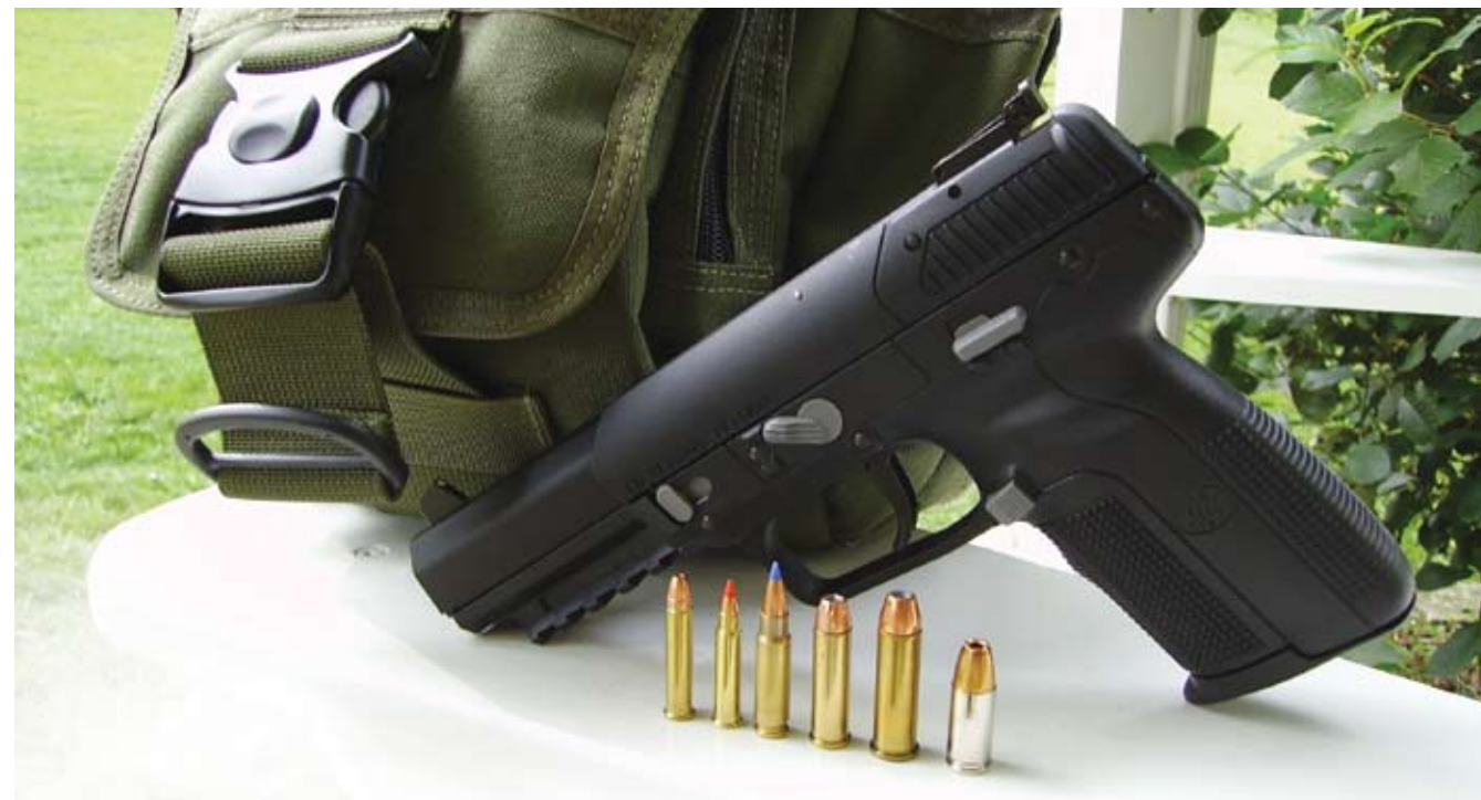
FiveseveN PISTOL WITH MAXPEDITION JUMBO S TYPE VERSIPACK AND FIVE ROUNDS THAT OPERATE WITHIN THE RANGE OF THE 5.7 X 28, FROM L TO R, 22 WRF MAGNUM WITH 40-GR. HP, .17 HMR WITH 17-GR. VMAX BULLET, 5.7 X 28 WITH 40-GR. VMAX BULLET, .32 H&R MAGNUM WITH 85-GR. JHP, 158-GR. .38 SPECIAL STANDARD VELOCITY JHP, AND 9MM WINCHESTER SXT 127-GR. +P+.
