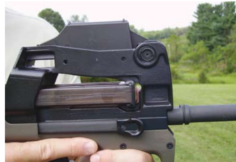
VIEW OF ONE OF TWO AMBIDEXTROUS BACKUP FRONT SIGHTS ON PS90. BLADE SITS DIRECTLY ABOVE ALLEN SCREW IN CIRCULAR ASSEMBLY TO THE RIGHT.
